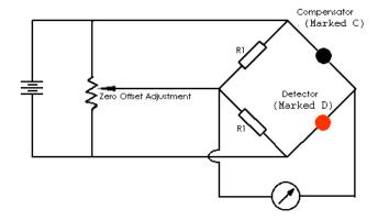
Note: The value R1 is arbitrary, since the function of R1 is to balance the bridge. 1  $k\Omega$  is suggested.
