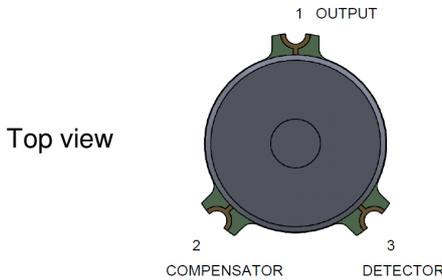
**A variant is available as a replacement for 3 Volt , 20 mm diameter, certified head sensors such as the VQ548ZD pellistor. The sensor is mounted onto pin holder socket and placed in a plastic head with the same VQ500 head dimensions.**
