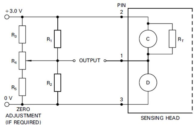
$$R_1 = R_2 = 500\Omega \text{ to } 10 \text{ k}\Omega$$
