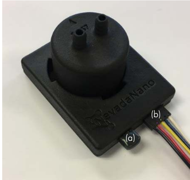
Figure 6 – Alternative communication configuration. The micro USB plug (a) is inserted prior to interfacing with the sensor via the 5-pin header (b)
