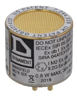
Dynament infrared gas sensors operate by using the NDIR principle to monitor the presence of the target gas. The sensor contains a long life tungsten filament infrared light source, an optical cavity into which gas diffuses, a dual temperature compensated pyroelectric infrared detector, an integral semiconductor temperature sensor and electronics to process the signals from the pyroelectric detector.
