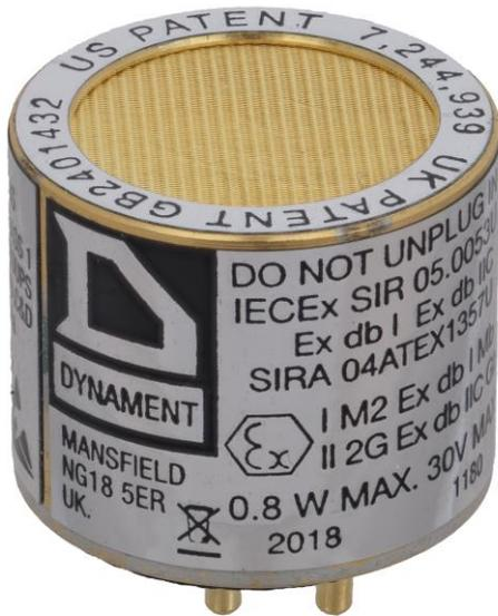
Dynamment infrared gas sensors operate by using the NDIR principle to monitor the presence of the target gas. The sensor contains a long life tungsten filament infrared light source, an optical cavity into which gas diffuses, a dual temperature compensated pyroelectric infrared detector, an integral semiconductor temperature sensor and electronics to process the signals from the pyroelectric detector.
